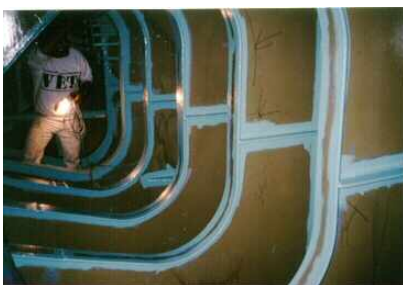
Fig 2. Ballast Tank showing multiple bays
